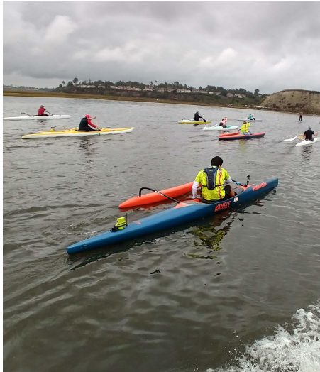
Figure 1: A blind paddler competing in a race with CoOP, a shared assistive technology for cooperative outrigger paddling. This was the first blind novice paddler participating in an OC1 race. Using CoOP, the paddler is responsible for all aspects of boat control except for steering. A sighted partner follows nearby to transmit directional changes to the canoe rudder.
