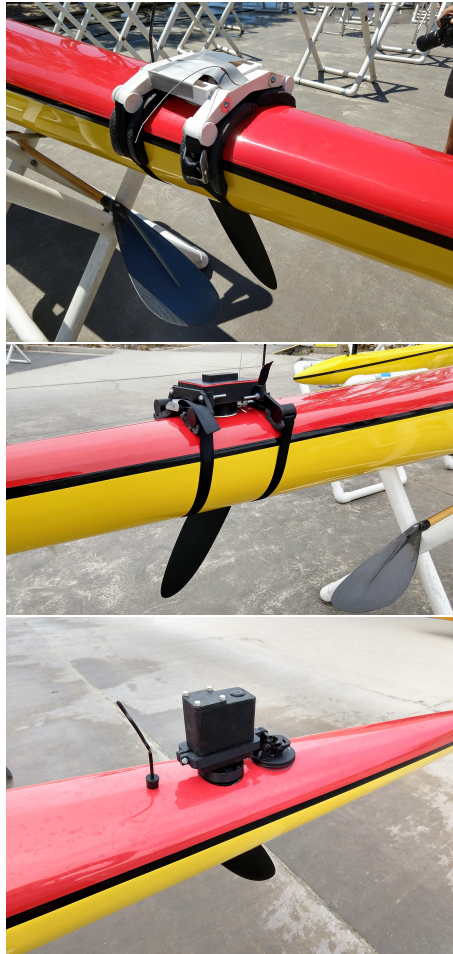
Figure 2: Various iterations of the CoOP-prototypes in order of improvement from top to bottom. The third iteration (bottom image) represents the combined insights from our findings and input from the paddling community.
